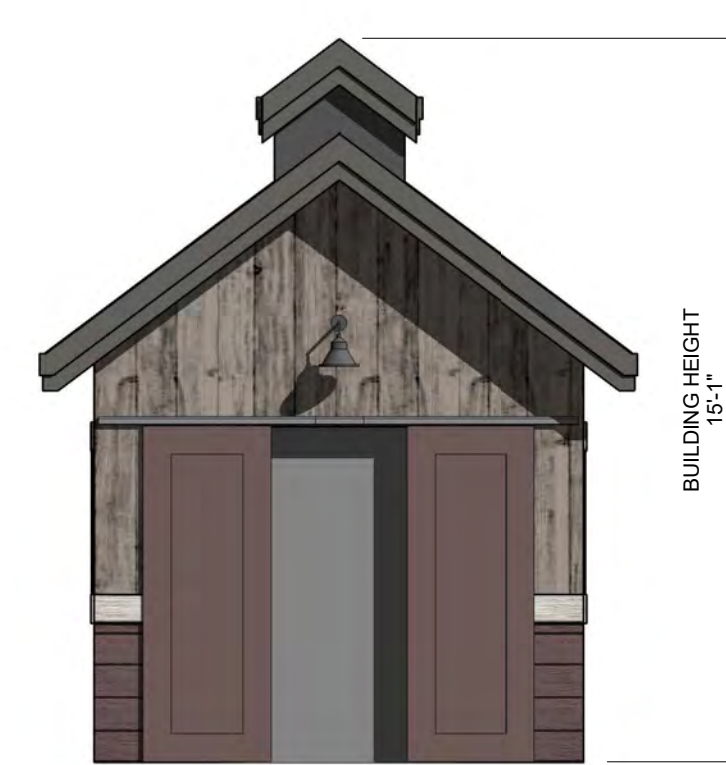
5 SOUTH ELEVATION - POTTING SHED 1/4" = 1'-0"
