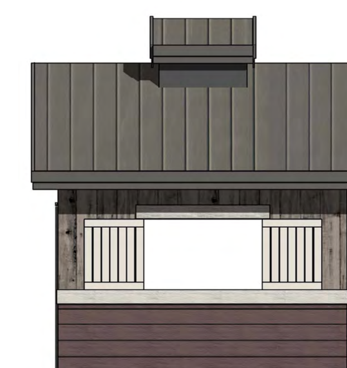
8 EAST ELEVATION - POTTING SHED 1/4" = 1'-0"
