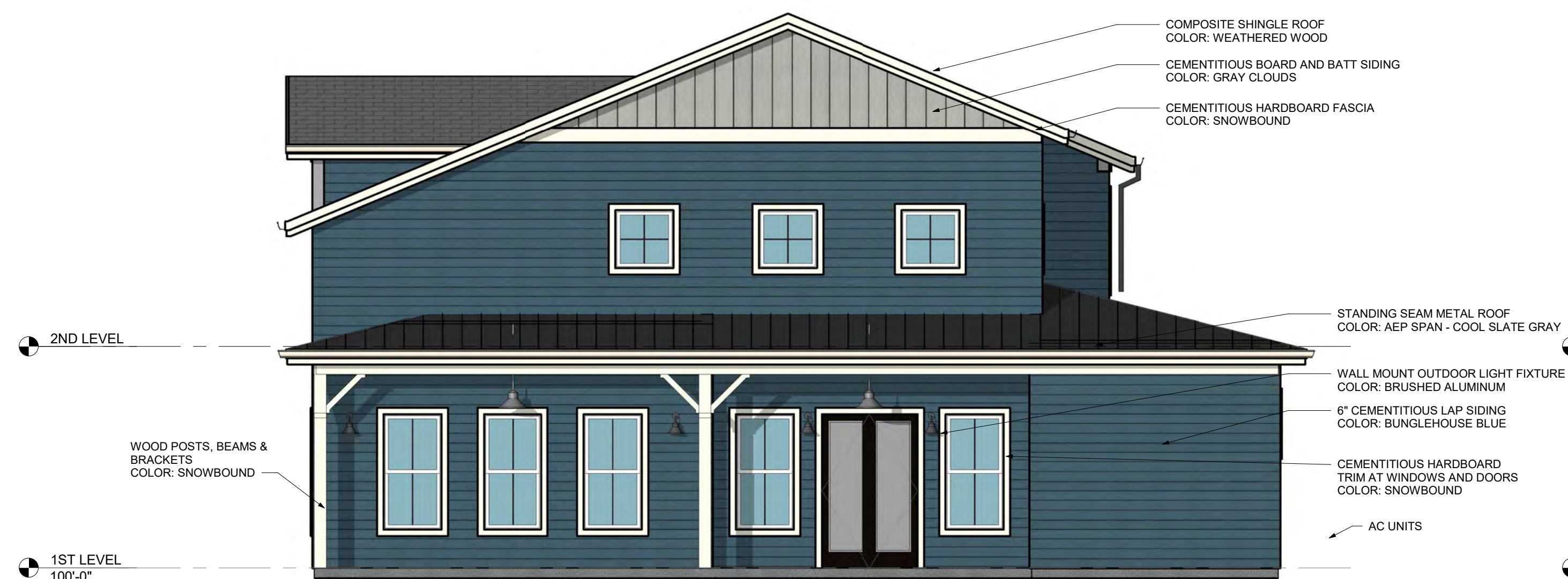
4 EAST ELEVATION 3/16" = 1'-0"
