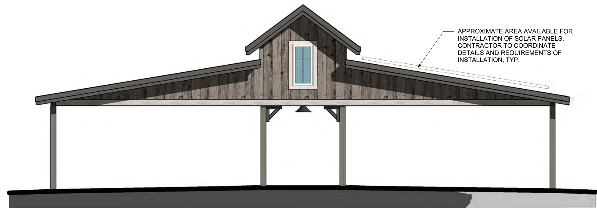
3 NORTH ELEVATION - PARKING STRUCTURE 3/16" = 1'-0"
